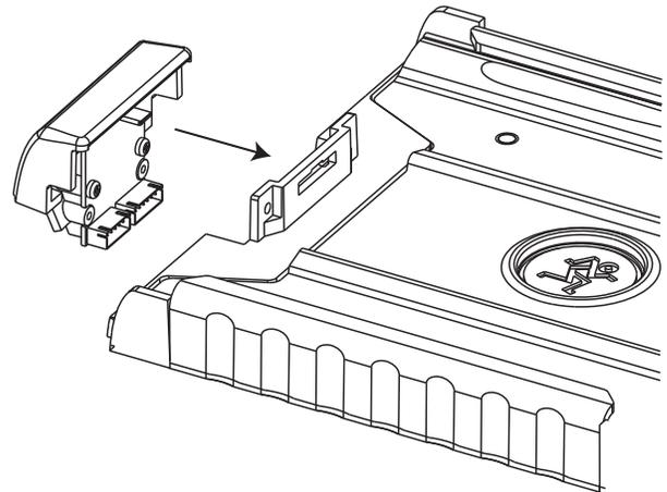
11. Now let's check your work. Slide the iPad down the tray until it mates with the dock connector and snaps into place, *but do not force it*. If it does not fit, continue on to step 12. If it is a great fit, jump forward to step 13.
