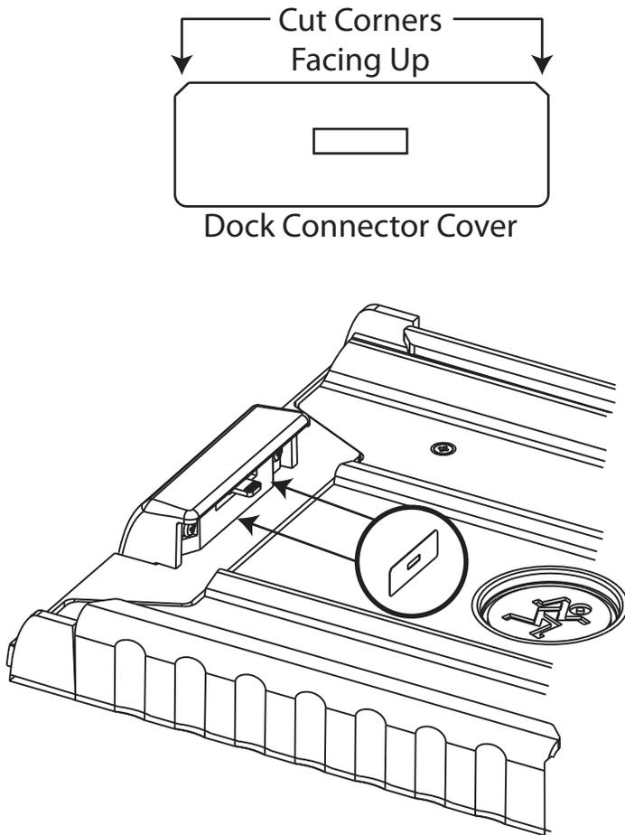
14. The hard part is done...let's finish it up! Place the entire tray assembly back into the mixer, making sure to first reattach the two cable assemblies that connect the iPad dock connector to the mixer.
