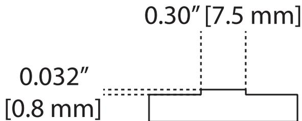
B. Verify the notch size by inserting the connector subassembly into the tray to be certain the notch is sized correctly. No plastic should touch the Lightning connector around the completed slot. Be sure there is no plastic protruding outward from the slot and that all burrs are removed.
