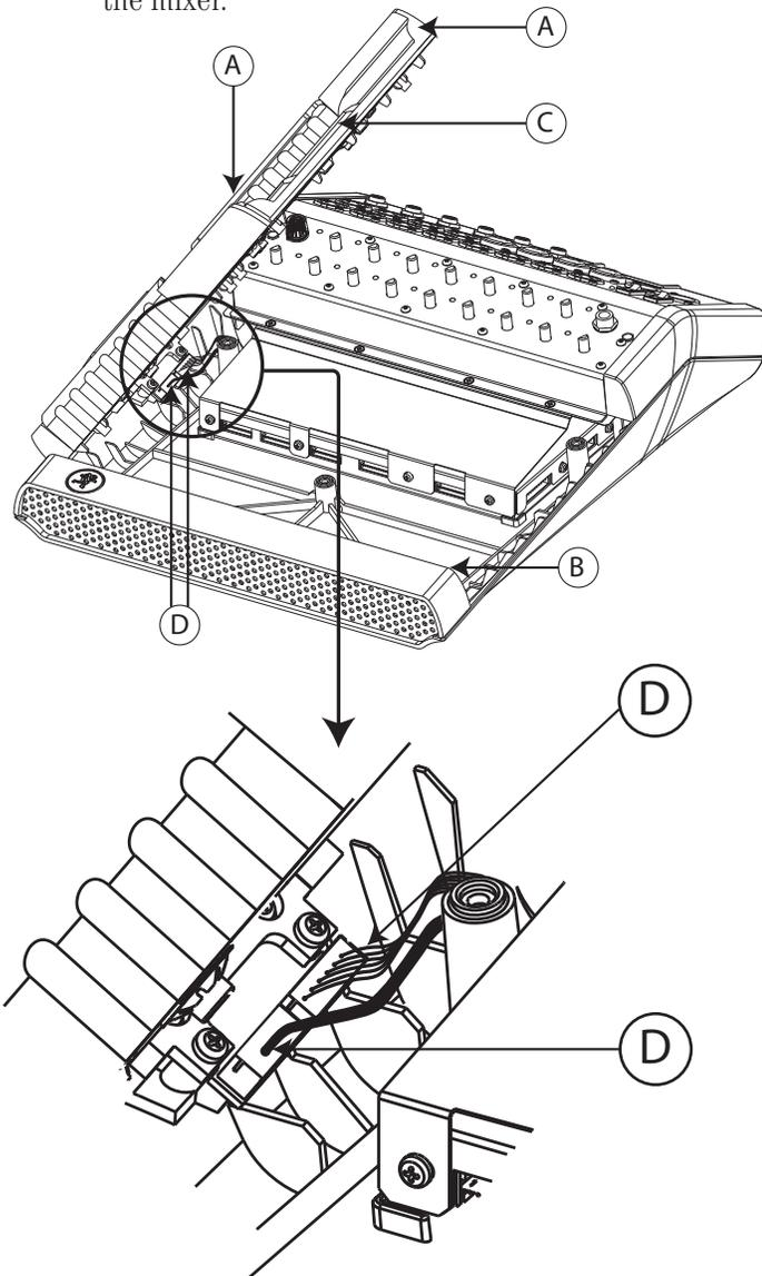
5. At this point, your goal is to remove the current iPad dock assembly from the tray assembly and replace it with the Lightning iPad dock assembly included with this kit.
